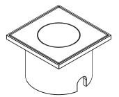
0.7 Cable + Connector Space Fixture Cable Bend is 0.5 From Bottom of Fixture
